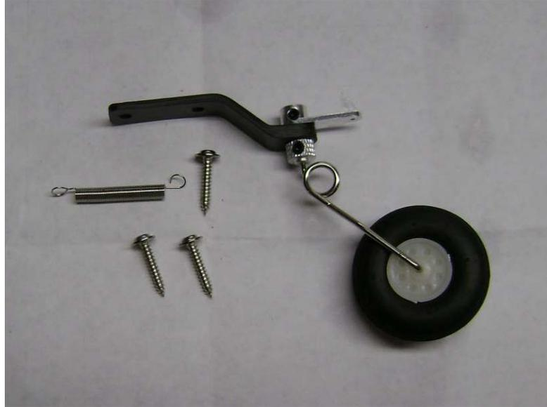
7. Center the tail wheel bracket on the rear of the fuselage. Screw the tail wheel assembly in place using the two supplied wood screws. Remove the screws and harden the holes with a drop of thin CA. Allow the CA to cure and then permanently install the tail wheel bracket. Install the rudder at this time using 4 CA hinges. Once the rudder is installed and the hinges have dried, use the third wood screw to attach the tail wheel spring as shown in the picture below.
