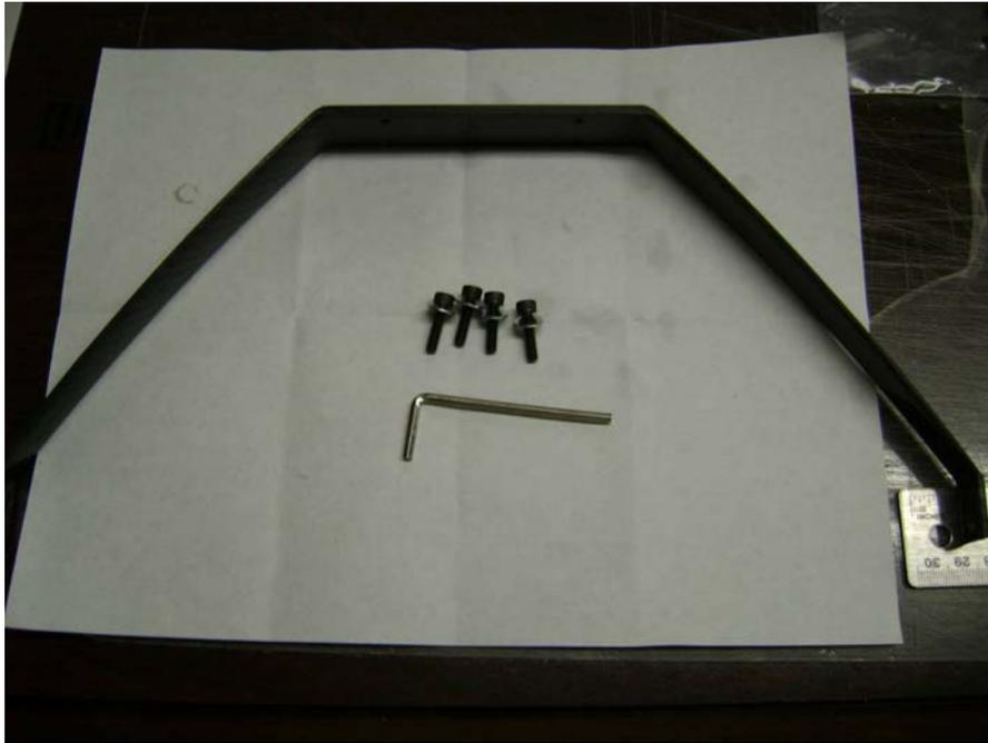
2. Bolt the main gear to the bottom of the fuselage using the supplied bolts. Use a small drop of thread-lock to secure the bolts in place.
