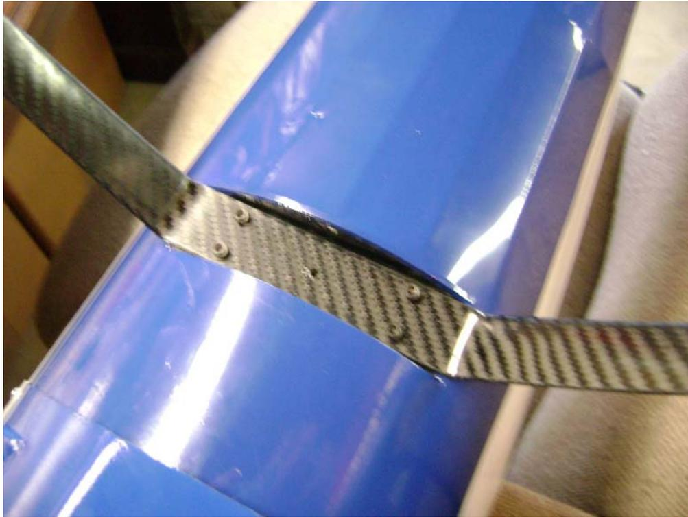
3. Once the main landing gear has been installed, install the cover over the main landing gear.
