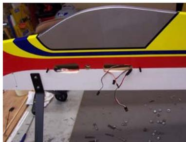
5. Finish installing the control linkages to all the surfaces with the supplied pushrods, clevises and ball links. The one longer control rod is for the rudder. Use proper geometry to assure optimal performance. Use the sub trim and end point adjustment features of your radio to match centering and max throws of both ailerons and elevators.
