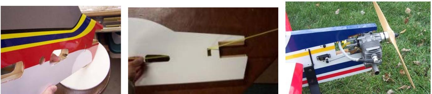
3. Install the aileron servos in the wing using extensions as required. Hint: Make a small cable clamp out of scrap balsa to help hold the end of the servo wire near the root of the wing.
