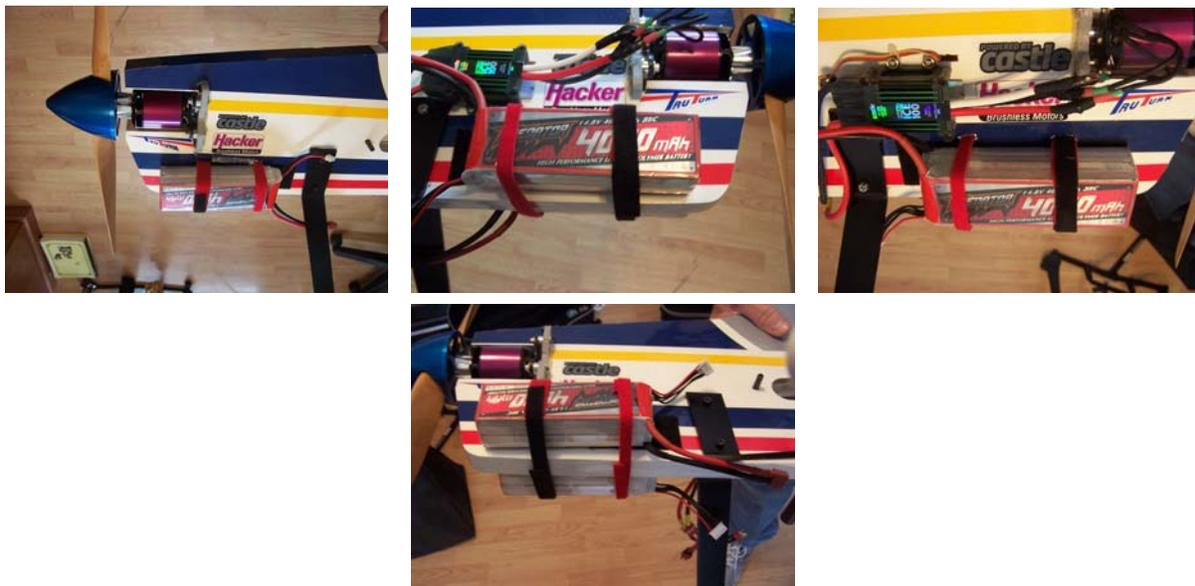
5. Mount the wings and install the lipo batteries under the motor. You can mount the ESC on either side of the fuselage in the available space behind the motor. Once you have found a location, drill holes through the fuselage for zip ties to secure the ESC. Use a Velcro strip to mount the ESC and the zip ties to secure it.
