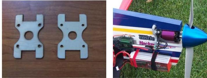
2. Now you have to make a decision as to how you are going to power the flight pack. If you are going to use a separate battery for the flight pack, install it in the battery hatch in the nose and follow the same steps to feed the battery lead back to receiver as the gas version. If you are going to use the BEC in the ESC to power the flight pack, then you will need to glue the battery hatch in place.
