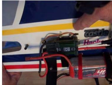
7. The lipo batteries can be moved front and aft along the Velcro strips to achieve the balance desired. The electric version balances in the same place as the gas version,
