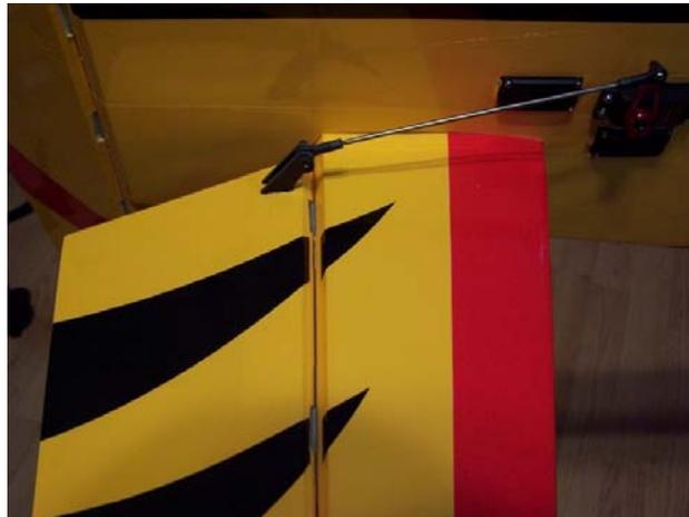
11. Now install the ailerons using the supplied hinges and the same technique as you did for the rudder and elevators. Double check the operation and tape the ailerons in place until the glue cures. Install the control horns in each wing likewise using the same technique as the previous surfaces.
