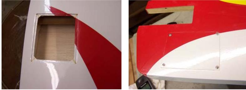
4. Be sure to seal any exposed wood with a thin coating of epoxy to prevent engine oil from soaking in. This is especially important around the engine compartment and servo openings with exposed areas. The Fusion ARF already has a factory applied coating of epoxy around the engine mounting area. If you need to widen the engine mounting rails be sure to reseal the wood.
