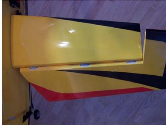
10. Now locate the carbon fiber horns (4) two for each side. Locate the two slots in the elevators and carefully remove the covering to expose the slot on the bottom only. Prepare the horns the same way as the rudder horns and glue in with epoxy or thin CA.
